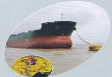
舟山无动力防台首艘单点系泊 Single point mooring of the first unpowered ship to against the typhoon in the city of Zhoushan.
